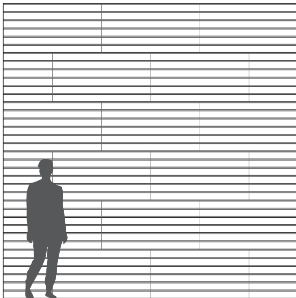
Troldtekt v-line 1way 6 installed in horizontal broken bond pattern.
