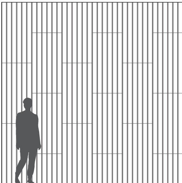
Troldtekt v-line 1way 6 installed in vertical broken bond pattern.
