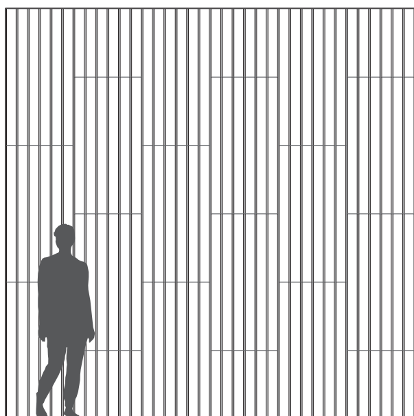
Troldtekt v-line 1way 6 installed in horizontal brick pattern.
