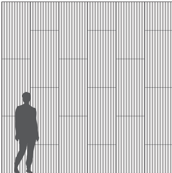
Troldtekt line installed vertically
