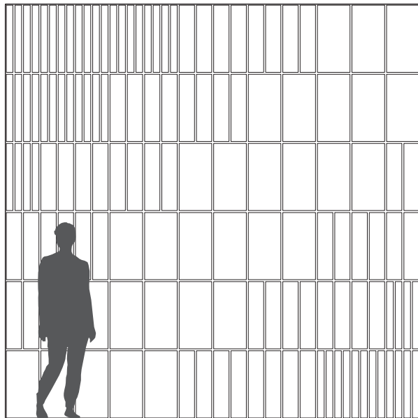
Troldtekt tiles installed in an alternative pattern
