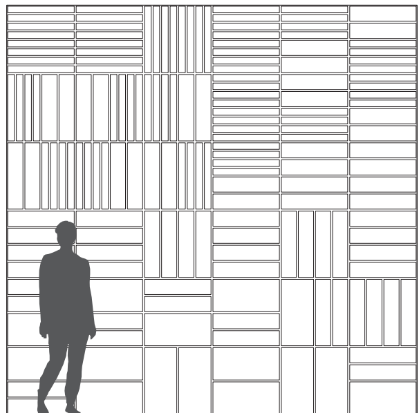
Troldtekt tiles randomly installed
