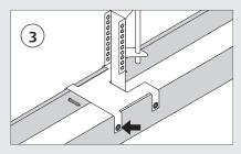
**3:** The quick-fit suspension bracket may be fixed to the main profile using screws in case of increased loads.
