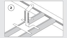
2: Hold a C60 profile with the opening facing upwards and fix a quick-fit suspension bracket at every hanger point. Assemble the C60 profiles longitudinally using C-connectors, and terminate the C60 profiles in the U-profile. If possible, divide the ceiling space to allow for adjustments of min. 300 mm on both sides.
