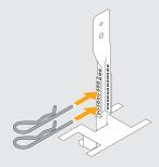
**2:** Secure the quick-hanger with nonius split-pins
