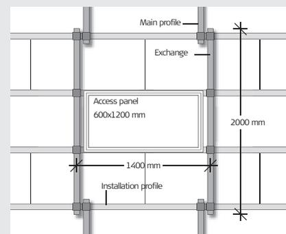
Load bearing replacement with 2 main profiles interrupted
