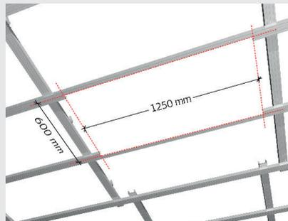
**B:** Profile system prepared for installation of the 1200 mm access panel.
