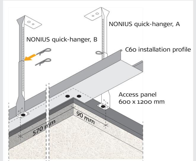
**C:** Hold the outer frame in position and secure it to the profiles with seven self-drilling screws. Then replace the access panel inside the outer frame.
