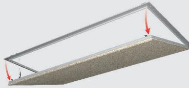
**2:** Once the frame is open, release the snap hook.
