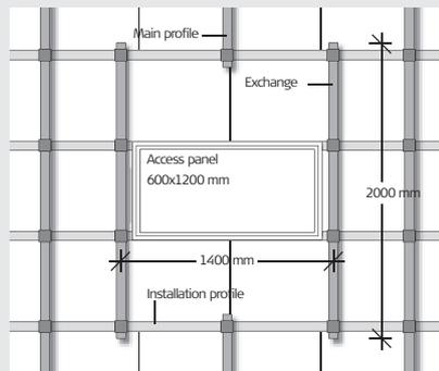
Load bearing replacement with 1 main profile interrupted
