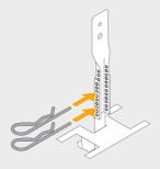
**2:** Secure the quick-hanger with nonius split-pins
