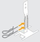
2: Secure the quick-hanger with nonius split-pins
