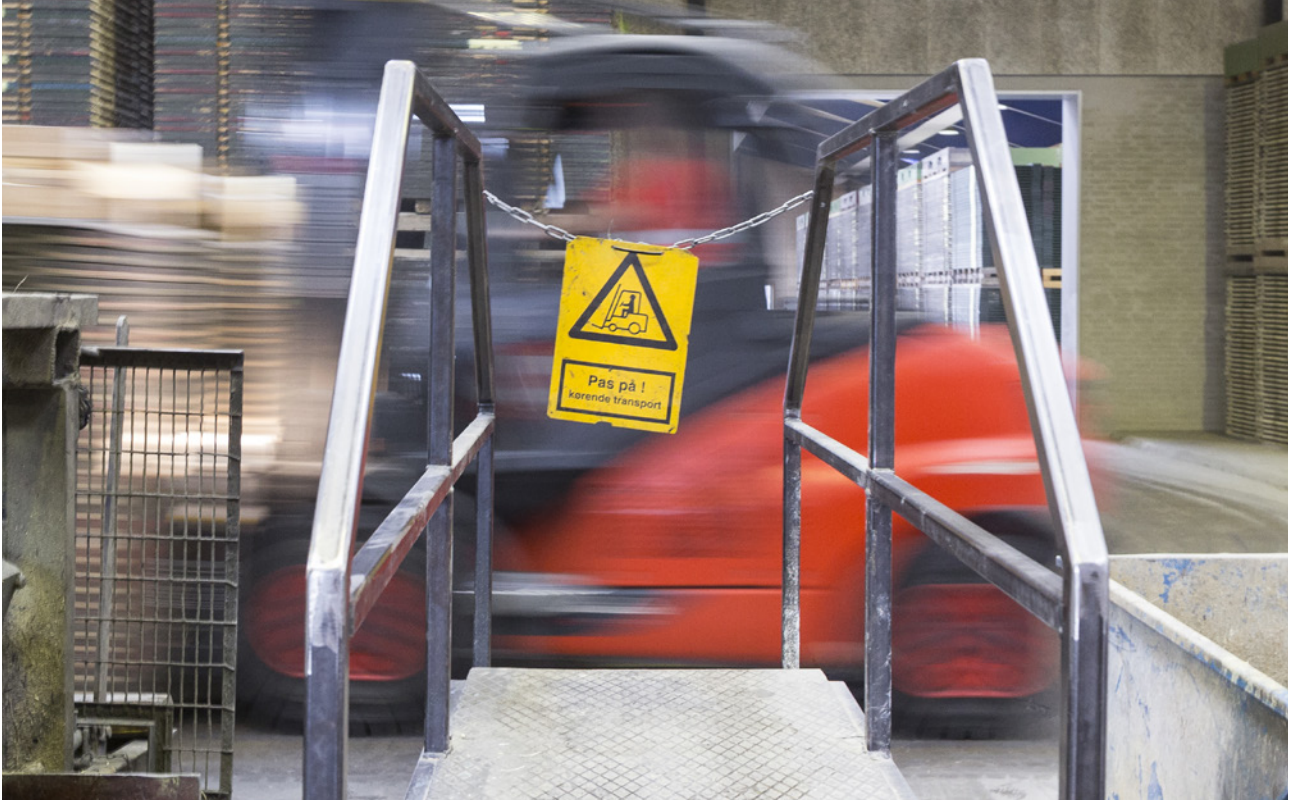
When driving with fork-lift trucks, the area is now completely cordoned off. The only exception to this is the maintenance and cleaning staff who first have to contact the truck driver.
