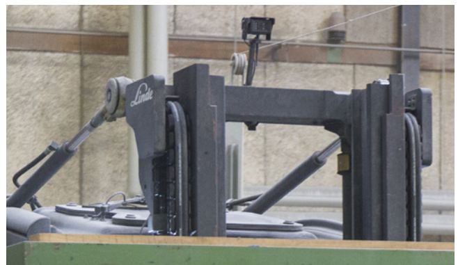
A camera has been installed on the truck so that the driver is better equipped to spots any hazards via a monitor in the cab.
