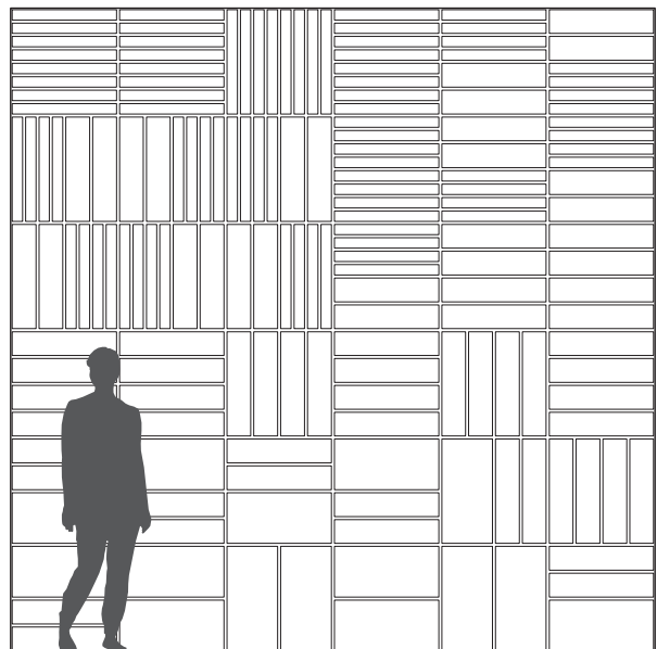
Troldtekt tiles randomly installed
